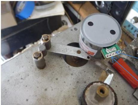
This is how I like to mount it so the wiring terminals are facing the front of the chassis. This one I use Gorilla Glue which is strong enough to fix a gate hinge on a metal post. Its not going anywere.
