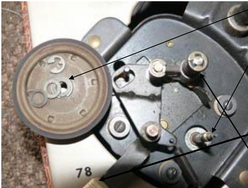
As shown, the clip has been removed and the wheel removed from its shaft.
