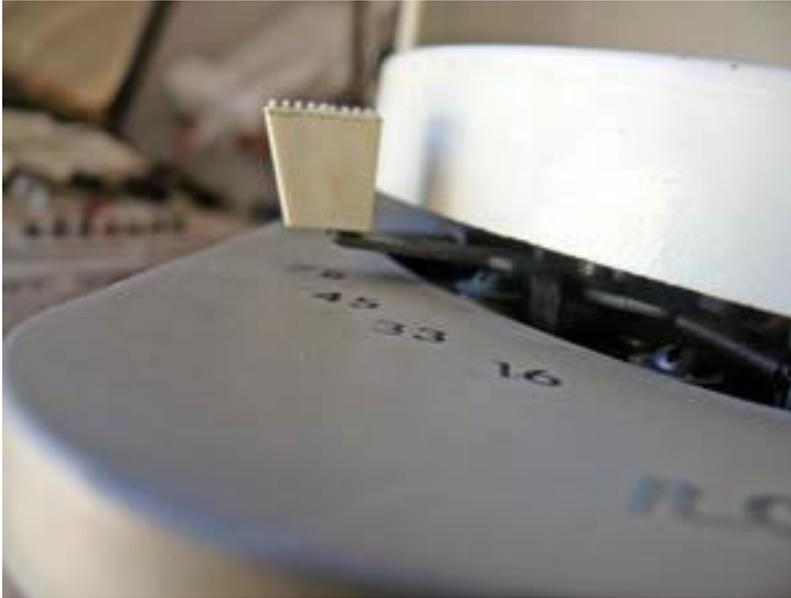
After everything and all clips are back in place, plug your player back into the wall and give it a spin (pardon the pun) If you lubricated the shifter mechanism, it should change speeds easier. If you cleaned the wheel sufficiently, you should be able to put your finger on the platter and it should continue spinning at any speed. As far as changing needles, most of these units used a spade lug needle. Look at that paper also on this site for instructions on its replacement. Good Luck.
