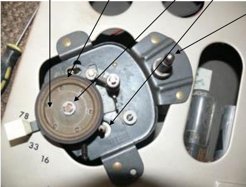
To the left or sometimes elsewhere is the speed changer. Like the transmission on a car, it changes the speed the drive wheel turns. The motor shaft which is "stepped" always turns at the same speed. As you move the shifter, it will move the drive wheel up and down on the stepped drive to run at a different speed. The stepper shaft and the rubber surface of the drive wheel must be very clean to keep good contact and not slip.
