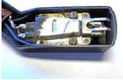
Many unrestored 45rpm record players have this old style Astatic cartridge and needle. It will tear up your 45s unless the needle is replaced regularly if it works at all. The best solution is to replace it during repair or restoration. There are many YouTube videos and sellers of kits, but I have put together a kit that takes all of the makeshift mounts and wiring obsolete.
