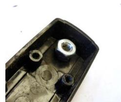
Start by gluing two hex nuts on the post in the front of the arm. They are necessary because the new assembly is lighter than the old one. Once they have "set up" use a good glue such as super glue to glue the modified bracket to the top of the arm .
