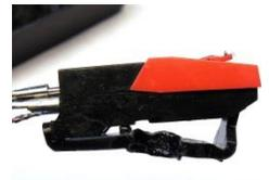
It is easiest to have the cartridge already in the holder when gluing it to the top of the arm, from the inside of course. Also have the enclosed wires with the installed female connectors in place too.
