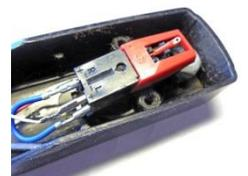
This is the unit glued in place in its bracket. Once the cement has hardened, it is easy to snap the cartridge out of its holder by prying the front clip away from the snap. It comes out as easy as putting it in. This makes service a "snap".
