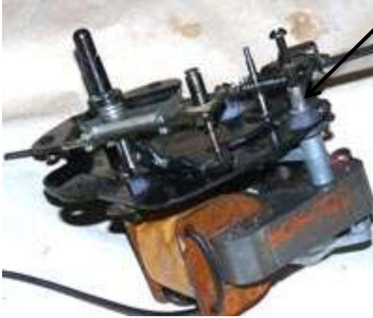
The screws are mounted from the top of the plate. Two are very long and go all the way through the motor bearings. Note the positions of the washer, the spacer and on the bottom bearing will be a lock washer and nut.
