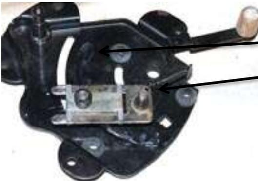
Also note the lubricated places of metal contact.
