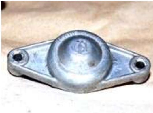
Identification can be made by looking at the bottom bearing on different motors. The Aluminum casting sports the GI logo and on the other side is the bronze bearing with a felt that should be saturated when oiling. This will be covered later
