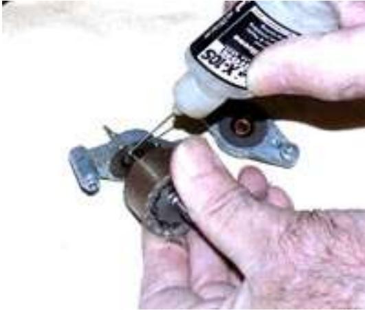
After a good cleaning with alcohol, inside each bearing is a felt. Saturate the felt with machine oil on both bearings and leave a small amount on the shaft.
