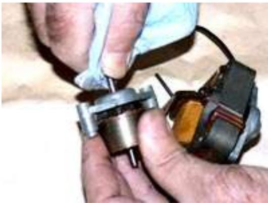
Using a paper towel or rag, clean the stepper portion of the upper motor shaft with alcohol. Leave no residue traces.
