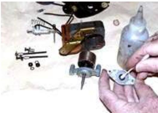
Use a cue tip and alcohol to clean the bearing and friction surfaces. Remove all traces of the old oils on both the top and bottom bearing
