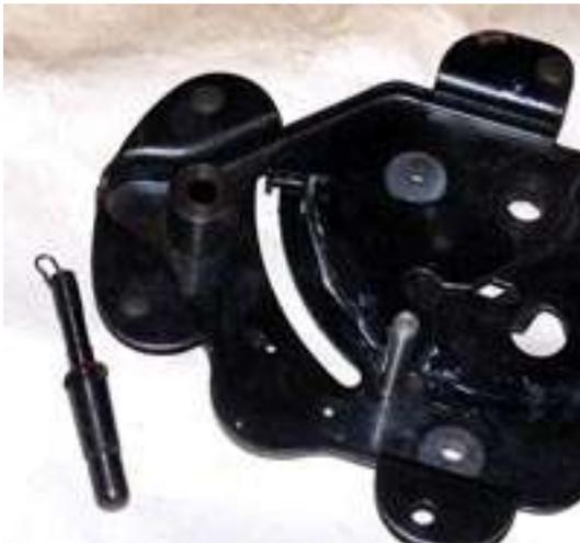
The center spindle should be removed by taking off the clip on the underside and pulling the spindle upward. I have had the lube used in these so hard I had to soak them with MEK to get them to release. Obviously the turntable platter did not turn in these cases. Clean the inside of the bearing with a cue tip and alcohol and also the entire spindle. Relube it and reinstall. Don't forget to use the clip to hold in firmly.
