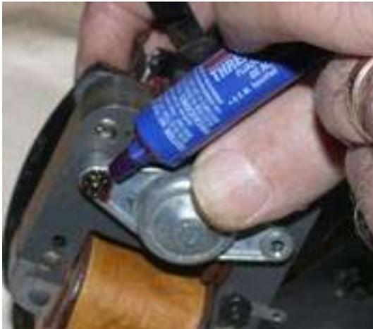
Once the screws are in place, on the bottom bearing use the locking washers and nuts. Use "Loctite" to make sure they do not vibrate loose. I know this sounds like a little "overkill", but experience has proven over the years that it will save you many hours of "re-do" down the line.
