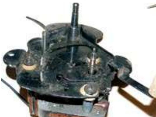
Do not be surprised if some parts do not move smoothly. The lubriplate used 50 years ago usually has turned to hard clay by now and may need a penetration liquid to soften it enough to remove some sliding parts.
