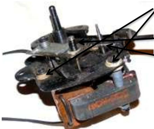
At this point you can see the deteriorated motor mounts. Three in all.
