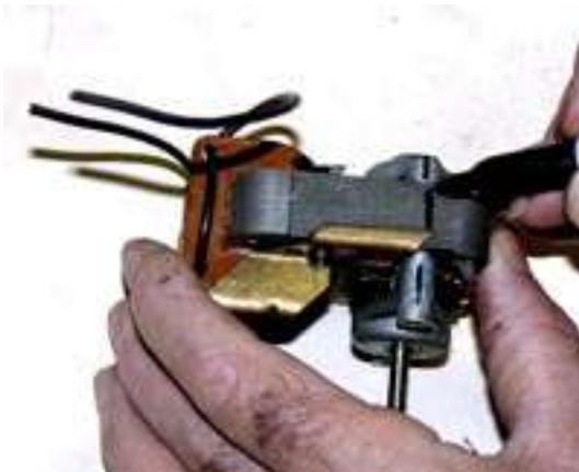
I always use a permanent marker to mark one side of the motor and upper and lower bearings. This enables easy reassembly without guessing what was top and bottom. As a synchronous motor, if the upper and lower bearing were switched, the motor would run backwards.
