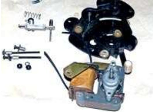
The GI motor has been removed from the motor plate. Note the rubber mounts condition. To the left of the motor are the screws, washers, spacers and nuts. Above them is the idler mount mechanism. A close look at the left side of the motor mount you will see the stepper that moves the idler up and down to match the steps on the motor shaft. Of course, on-line, you can click on the pictures to get a larger view.
