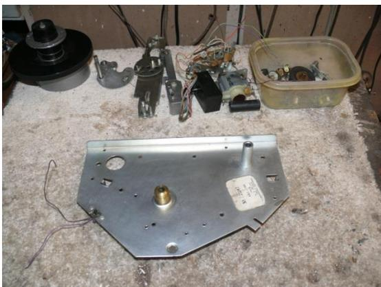
After disassembly, the parts are dipped cleaned and plated as necessary. This chassis is ready for re-assembly..
