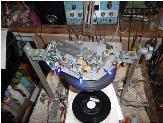
Lights are mounted, motor in place and electronics for stereo. The chassis is then played continuously for 3 or four days to show any deficiencies that need attention. It is then mounted in its case and played another day before shipping. Lights are installed according to the customer. This one wanted blue LED's.
