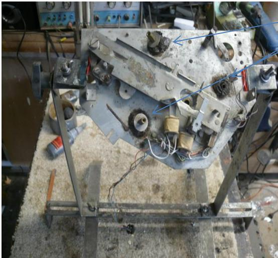
Most units received have not been used for years and the lubriplate has turned to stiff glue like substance. Many are frozen tight. This unit will be completely refurbished like new.
