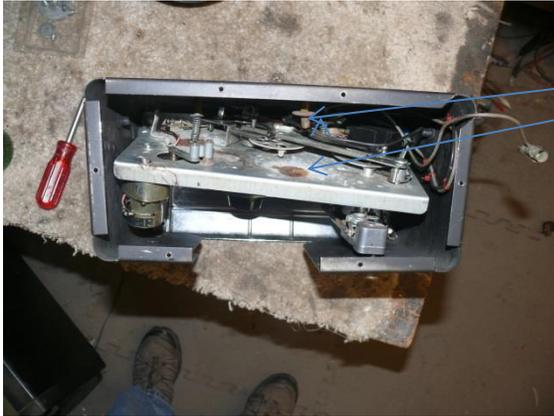
An "as received" ARC. Note the broken suspension spring, stretched rear spring with no "shock" and the general condition of the chassis and attached components. This unit is in for a general refurb and conversion to stereo.
